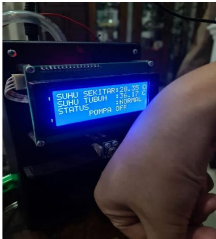
Gambar 8. Pengujian sensor GY-906 Suhu normal
